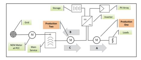
To illustrate, imagine a NEM paired storage system under an Option 2 metering configuration that serves a 10-kW load and has a 10-kW PV system and 5-kW battery storage system installed with a single DC inverter. In the example below, across five hypothetical hours of the day, the NEM paired storage system only charges the storage system from the NEM generator, which will be evident in the B and C registers on the meter. The A + B - C value would read 20 kWh for the day.
